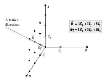
**Figure 145** A lattice direction. The vector  $\vec{a}_{\tau}$  is the shortest one in this direction.
