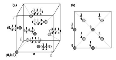
**Figure 97 (a)** Positions of the eight atoms within the cubic unit cell of the diamond structure. The coordinates are expressed in units of a. (b) Projection of atoms on the cell base. The fraction nearby the projection of an atom represents its coordinate in the  $\vec{c}$  axis.
