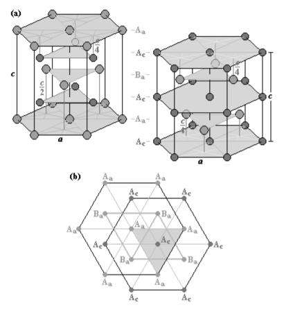
**Figure 116** (a) Two hexagonal prisms for the NiAs structure: one with anions at the vertices and another one with cations at the vertices. (b) Projection of the centers of ions belonging to each hexagonal prism on the hexagonal base. We can observe that the triangles defined by the ions from the  $B_a$  layer have in each case from (a) different orientations with respect to the hexagonal prism base.
