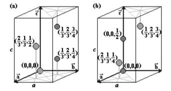
**Figure 120** (a) and (b) show the positions of ions belonging to the unit cells from Figs. 119a and 119b, respectively. The coordinates are expressed in units of a and c.
