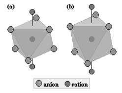
**Figure 115** Octahedrons defined by anions that are the NNs of a cation (a) in the NiAs compound and (b) in the ideal NiAs structure. In this figure we also show the two nearest cations to the cation placed in the center of each octahedron.
