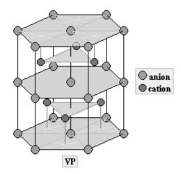
Figure 121 Anti-NiAs structure shown on the example of the VP compound.
