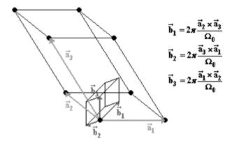
**Figure 135** Primitive unit cell of the reciprocal of the triclinic lattice. In the figure, we show also the primitive unit cell for the direct lattice.
