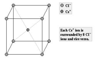
Figure 130 Conventional unit cell for cesium chloride.
