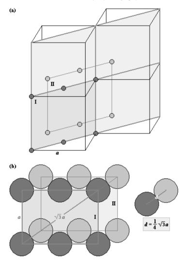
Figure 94 (a) Comparison of the distribution of atoms from vertices and faces of the cubic unit cells with those from their body diagonals in the diamond structure. (b) Cross sections of atoms (considered hard spheres) from (a) are shown. In this figure, the equivalency between the relative distributions of atoms of each type (those from vertices and faces of the cube and those from its diagonals) is visualized.
