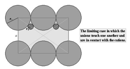
**Figure 102** A plane defined by two body diagonals of the cubic unit cell for the zinc blende structure shown in Fig. 100. In the figure, we show the limiting case in which the anions, represented by larger circles, touch one another and are in contact with the cations (smaller circles).
