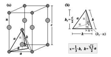
**Figure 112 (a)** A regular tetrahedron, defined by Zn cations, located inside a hexagonal unit cell for the wurtzite structure of ZnS. **(b)** A vertical cross section of the tetrahedron shown in (a). See text for detailed explanation.
