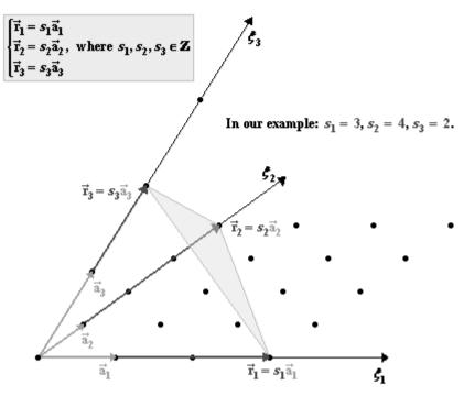
**Figure 141** Three-dimensional crystal lattice generated by the primitive translation vectors  $\vec{a}_1$ ,  $\vec{a}_2$ ,  $\vec{a}_3$ . The lattice plane shown in the figure intersects the axes  $\xi_1$ ,  $\xi_2$ ,  $\xi_3$  in the lattice points.
