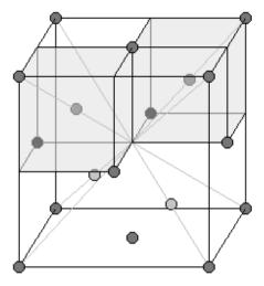
In the center of the small cube that represents an eighth of the cubic unit cell there is an atom marked with  $\circ$ . The unit cell is composed of eight small cubes, four of which have an atom in the center.
