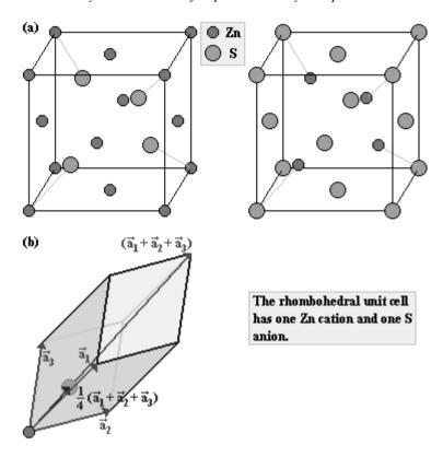
**Figure 103 (a)** Two cubic unit cells for the zinc blende structure of ZnS: one with Zn cations and the other one with S anions at the vertices. **(b)** A rhombohedral unit cell for the zinc blende structure with the two ions belonging to it.
