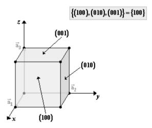
**Figure 144** Three lattice planes in the sc lattice that are equivalent by symmetry of the lattice.
