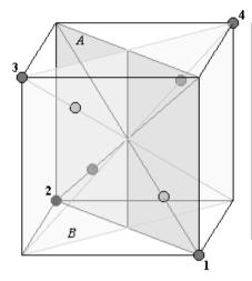
The 4 body diagonals of the cube (which represents the cubic unit cell of the diamond structure) define two vertical planes as shown in the figure. On the plane A there are two  $\circ$  atoms. These atoms are located on the diagonals, at a distance equal to 1/4 of their longitudes from vertices 1, 2 of the bottom base of the cube. Likewise, two atoms are located on plane E, but now equally distant from vertices 3, 4 of the upper base.
