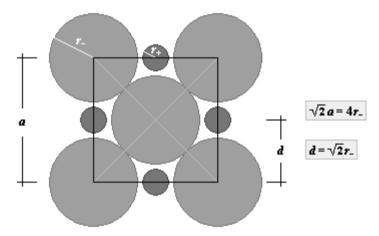
**Figure 129** The same plane as in Figs. 127 and 128, but now the smaller ion is too small to make contact with larger ions and as a consequence the ion located in the center of the cube face makes contact only with its NNNs (large spheres). The NN distance,  $d = \sqrt{2}r_-$ , is defined only by the radius of the larger ion.
