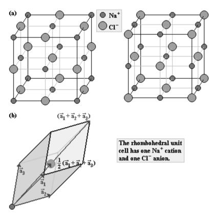
**Figure 124** (a) Two cubic unit cells for the structure of sodium chloride: one with Na<sup>+</sup> cations at the vertices and the other one with Cl<sup>-</sup> anions at the vertices. (b) A rhombohedral unit cell with two ions (one anion and one cation), which is the smallest unit cell that reproduces the NaCl structure.
