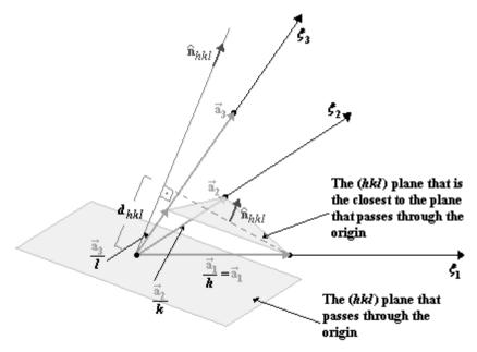
**Figure 150** Two consecutive (hkl) planes. The direction orthogonal to these planes, defined by versor  $\hat{\mathbf{n}}_{hkl}$ , is shown. The distance,  $d_{hkl}$ , between these planes is also indicated.
