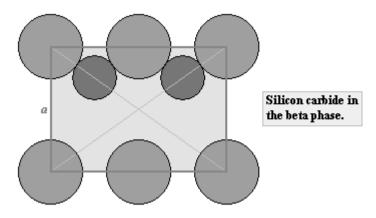
**Figure 101** Cross section from Fig. 100 of the cubic unit cell for silicon carbide in the beta phase. Larger circles correspond to the cross sections of Si atoms and the smaller ones to the cross sections of C atoms.
