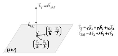
**Figure 149** The direction given by the vector  $\vec{\mathbf{b}}_{hkl}$  in the reciprocal lattice is orthogonal to the family of (hkl) direct lattice planes.
