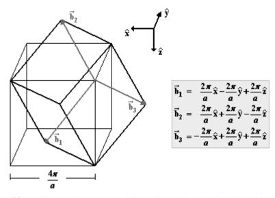
**Figure 138** Primitive rhombohedral unit cell for the *bcc* reciprocal lattice. The cell is defined by primitive translation vectors  $\vec{b}_1$ ,  $\vec{b}_2$ ,  $\vec{b}_3$  with coordinates given in the figure.
