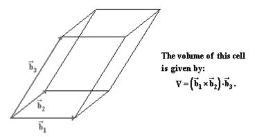
Figure 134 The unit cell of a reciprocal lattice defined by the primitive translation vectors  $\vec{b}_1, \vec{b}_2,$  and  $\vec{b}_3$ .
