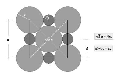
**Figure 127** The plane of a face of the NaCl cubic unit cell with the cross sections of 9 ions considered hard spheres. The large ion, located in the center of the face, makes contact with its NNs (small spheres) and also with the NNNs (large spheres). The NN distance, d, is equal to the sum of the ionic radii,  $r_- + r_+$ .
