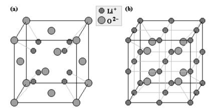
**Figure 106** Cubic unit cells of  $\text{Li}_2\text{O}$  which crystallizes in the anti-fluorite structure. In the cube vertices are placed  $\text{O}^{2-}$  anions in (a) and  $\text{Li}^+$  cations in (b).
