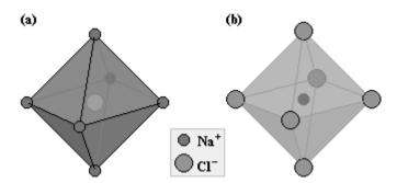
**Figure 123** The structure of NaCl. (a) Regular octahedron defined by Na<sup>+</sup> cations with the Cl<sup>-</sup> anion in its center. (b) Nearest neighbors of a Na<sup>+</sup> cation at the vertices of a regular octahedron.
