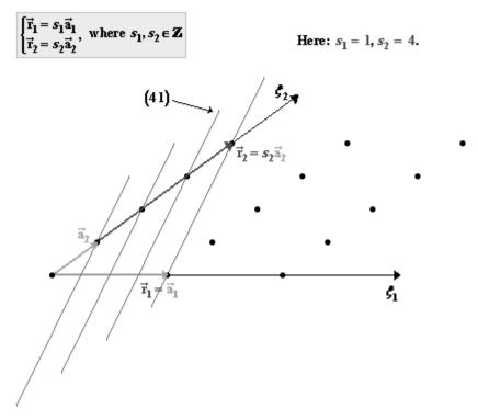
**Figure 154** Two-dimensional crystal lattice generated by the primitive translation vectors  $\vec{a}_1$ ,  $\vec{a}_2$ . In the figure four consecutive (41) lattice planes are shown.
