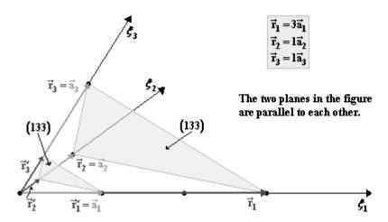
**Figure 147** Two (133) lattice planes in a lattice generated by the primitive translation vectors  $\vec{a}_1$ ,  $\vec{a}_2$ ,  $\vec{a}_3$ .
