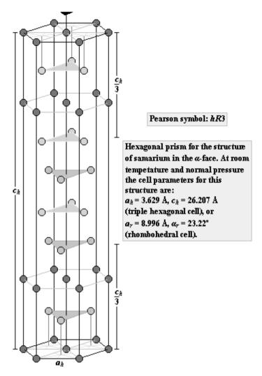
**Figure 98** Hexagonal prism for the  $\alpha$ -Sm structure.
