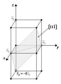
**Figure 142** A complementary figure to Fig. 140d. In this figure is indicated the lattice point where the  $(11\overline{1})$  plane crosses the z axis defined by the translation vector  $\vec{a}_3$ .
