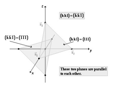
**Figure 143** The (111) and  $(\overline{1}\overline{1}\overline{1})$  planes in the *sc* lattice.
