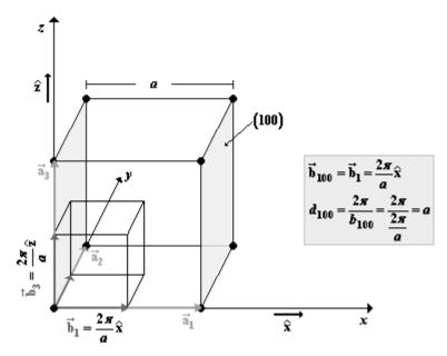
**Figure 151** The (100) planes which include two cube faces that are parallel to each other in the *sc* lattice. The cubic unit cell defined by primitive translation vectors  $\vec{\mathbf{b}}_1$ ,  $\vec{\mathbf{b}}_2$ ,  $\vec{\mathbf{b}}_3$  of the reciprocal lattice is also shown. The translation vector  $\vec{\mathbf{b}}_{100} = \vec{\mathbf{b}}_1$  is orthogonal to the (100) planes.
