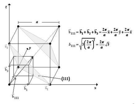
**Figure 152** The cubic unit cells of the *sc* direct lattice and the reciprocal to it. The vector  $\vec{b}_{111}$  of the reciprocal lattice is orthogonal to the (111) planes in the direct lattice.
