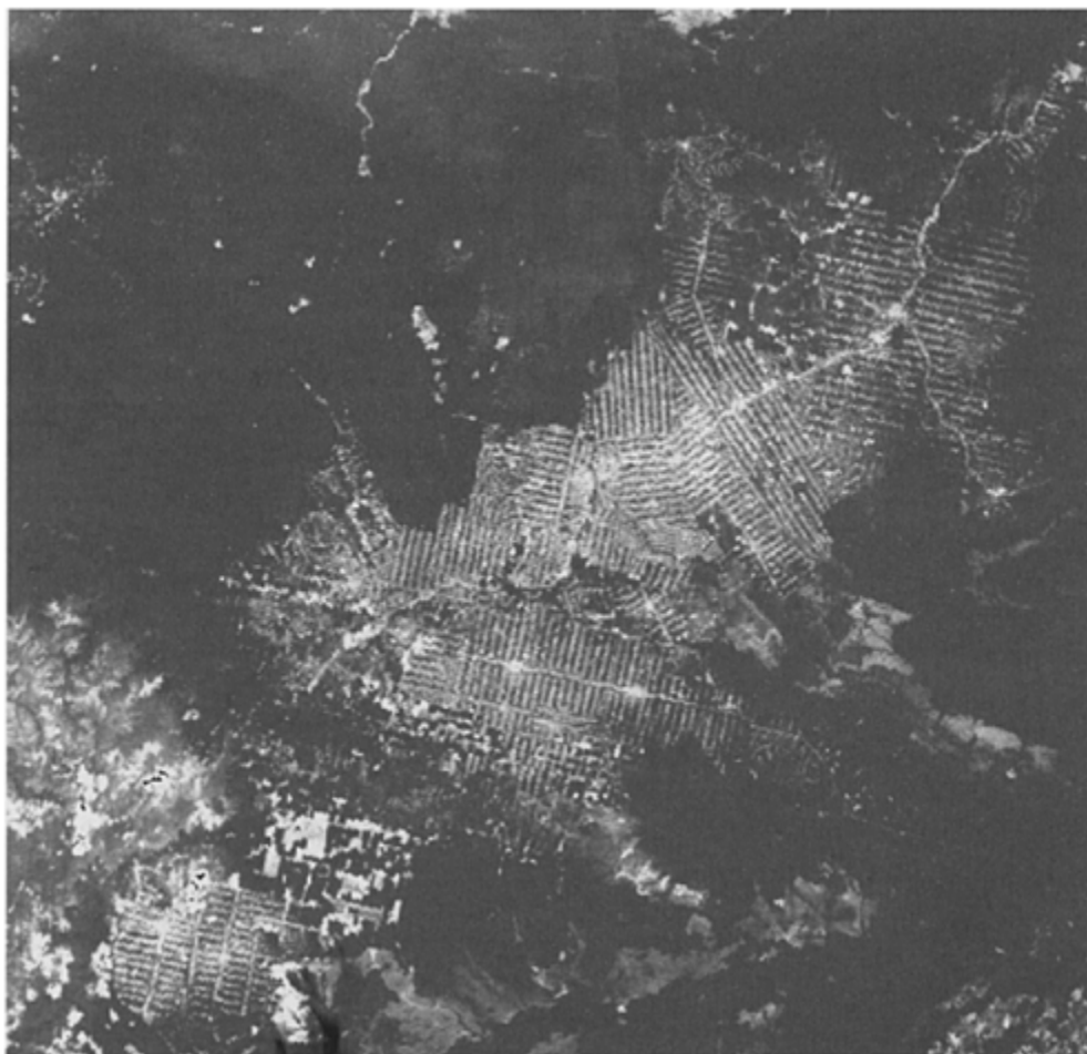
Plate 3.1 Deforestation of the Brazilian rainforest as shown by thermal RS imaging. This is an 11\ \mu\text{m} daytime image, 28 August 1991, covering an area of 512 \times 512\ \text{km} . The cleared areas show up brighter than the surrounding vegetation because they can be up to 4\ \text{K} warmer during the day.
