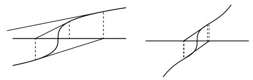
A milder form of non-convergence can occur if at the root the curvature changes sign and is large, as in the second graph. This can lead to a limit cycle where the iteration simply oscillates from one side of the root to the other without going anywhere. As I said earlier this doesn't always work.
