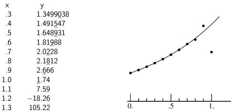
Everything is going very smoothly for a while, though the error is creeping up. At around x=1, the numerical solution goes into wild oscillation and is completely unstable. The reason for this is in the coefficients -4 and +5 of y(-h) and y(-2h). Small errors are magnified by these large factors. (The coefficients of y' are not any trouble because of the factor h in front.)
